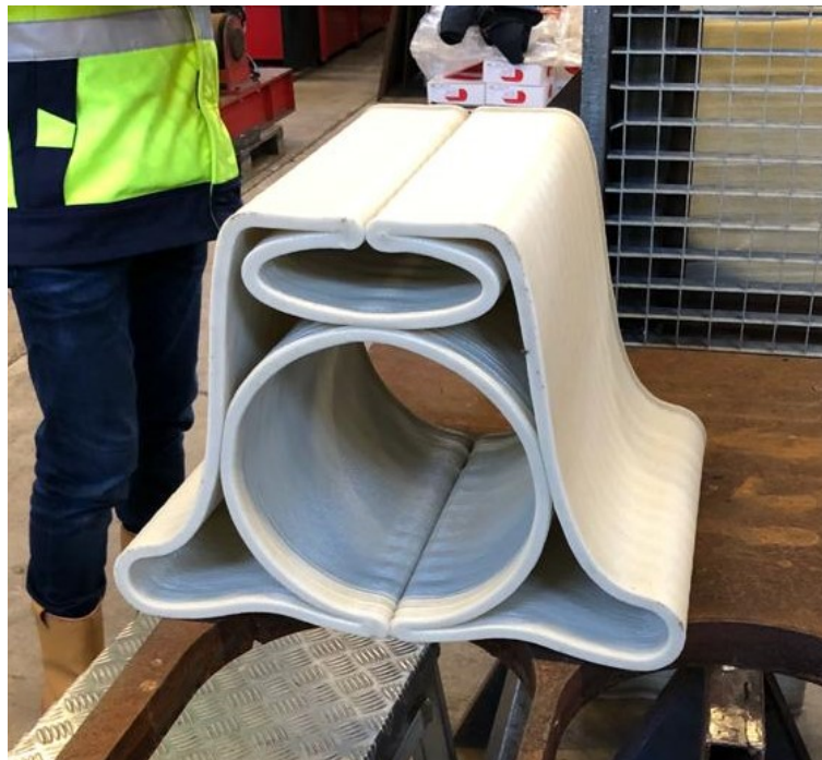
3D printed biocomposite fender profile for SeaBioComp project © Poly Products
